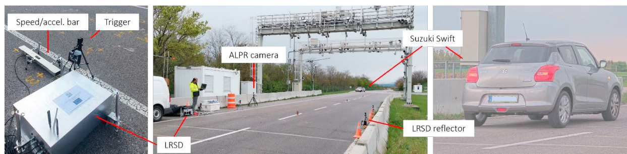
Figure 2. On-road test at Teesdorf, Austria, of a Suzuki Swift mil-hybrid gasoline Euro 6d passenger car.
