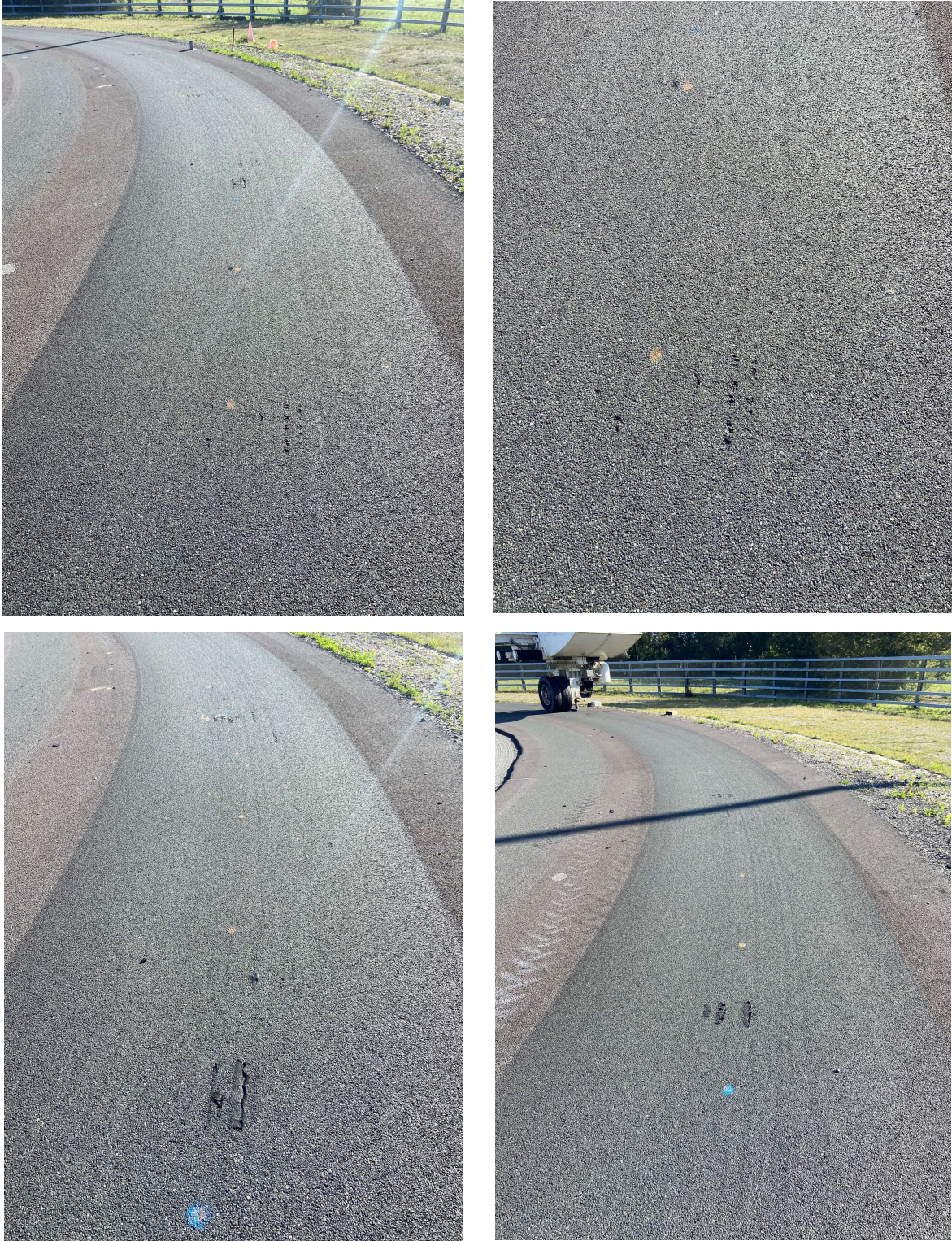
Figure 44. Photographs of the experimental peri-urban mixture asphalt after 1 million load cycles
