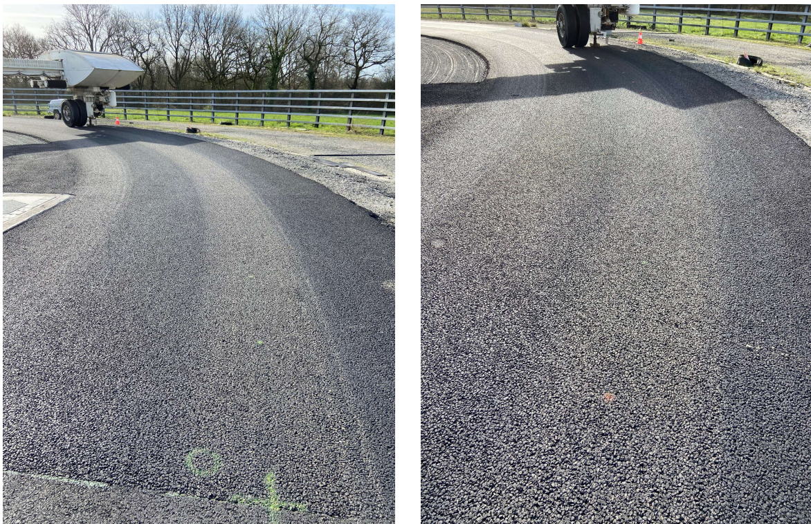
Figure 29. Photograph of the reference porous asphalt at 200 000 load cycles
