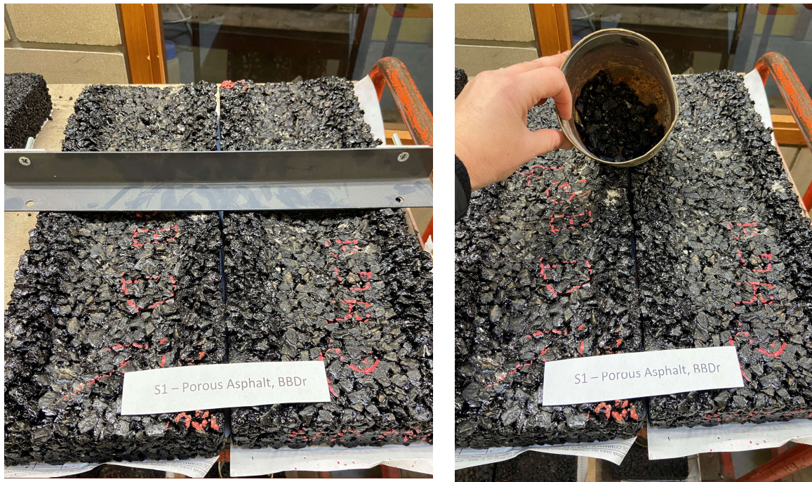
Figure 16. Porous asphalt specimens (S1) after the rutting test
