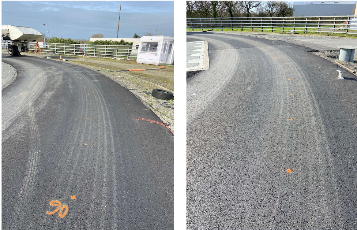
Figure 32. Photograph of the BBSG reference mixture asphalt at 200 000 load cycles
