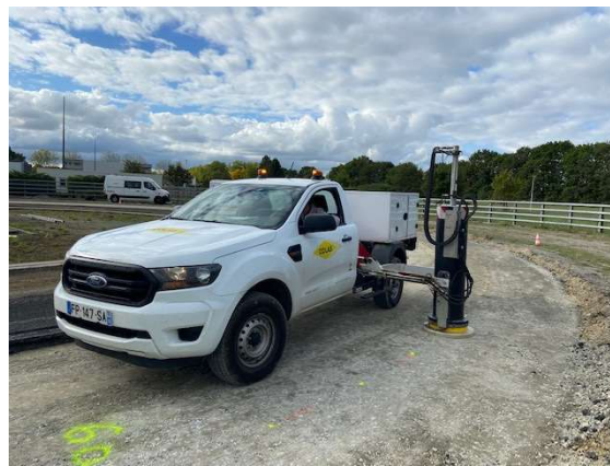
Figure 14. Measurement of bearing capacity (top of UGM) with dynamic plate load
