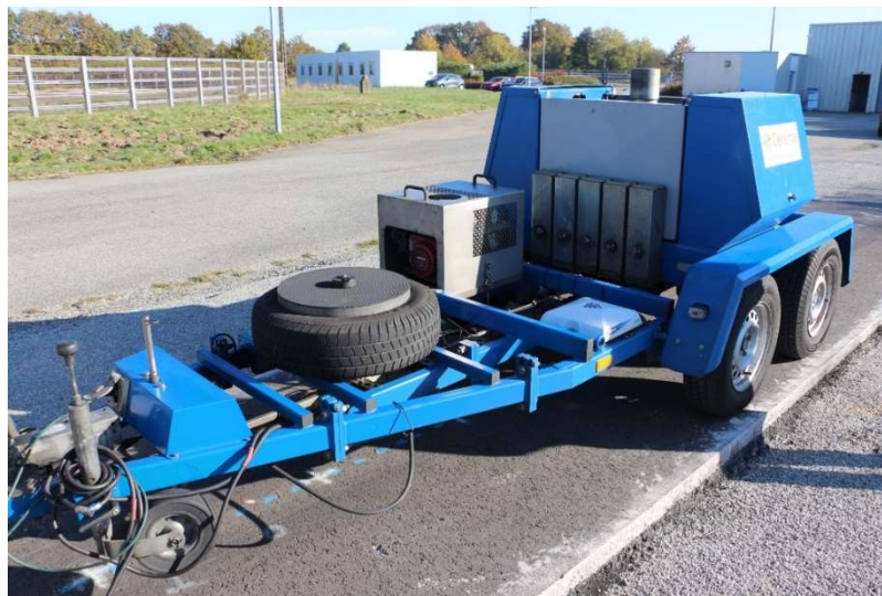
Figure 22. Falling weight deflectometer
