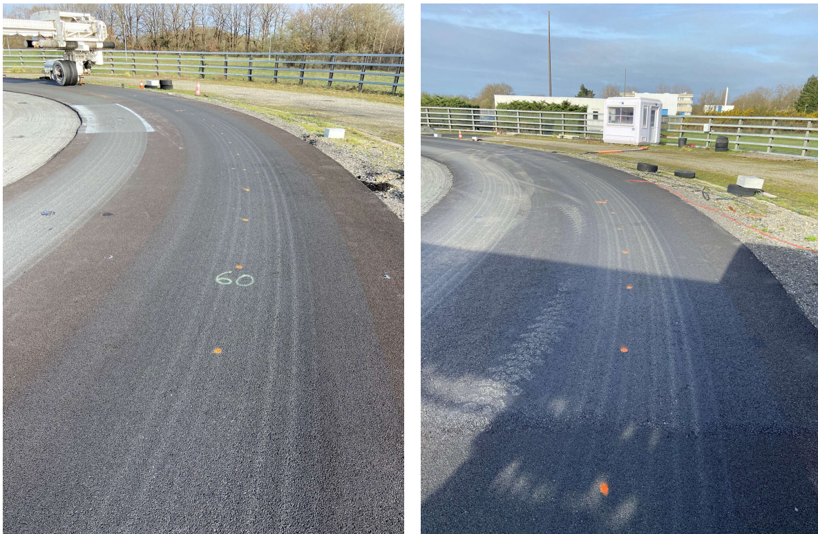
Figure 31. Photograph of the urban mixture asphalt at 200 000 load cycles
