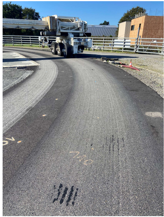
Figure 46. Photographs of the reference BBSG asphalt after 1 million load cycles
