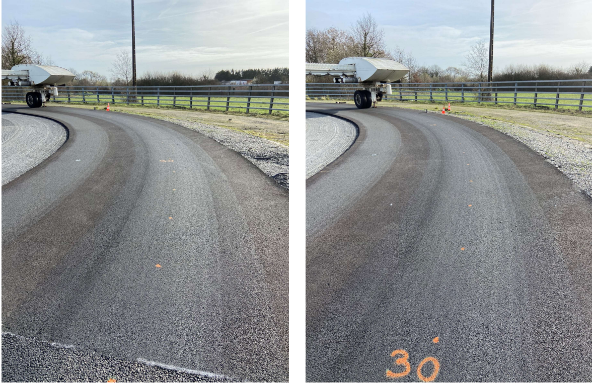
Figure 30. Photograph of the peri-urban mixture asphalt at 200 000 load cycles
