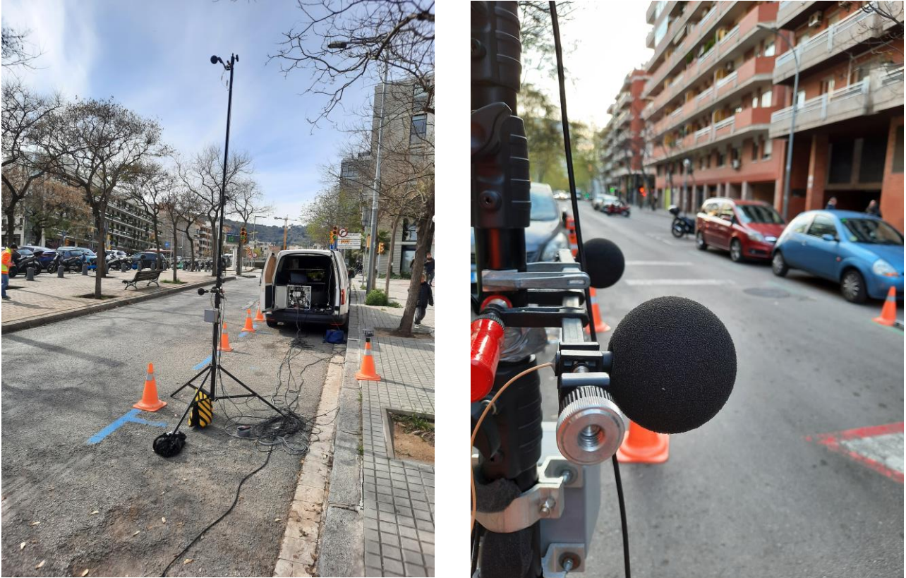
Figure 1: Microphone array mounted on a pole, left: vertical microphone pair and speed radar (below), right: horizontal microphone pair. Test setup in Barcelona, Spain, April 2022.
