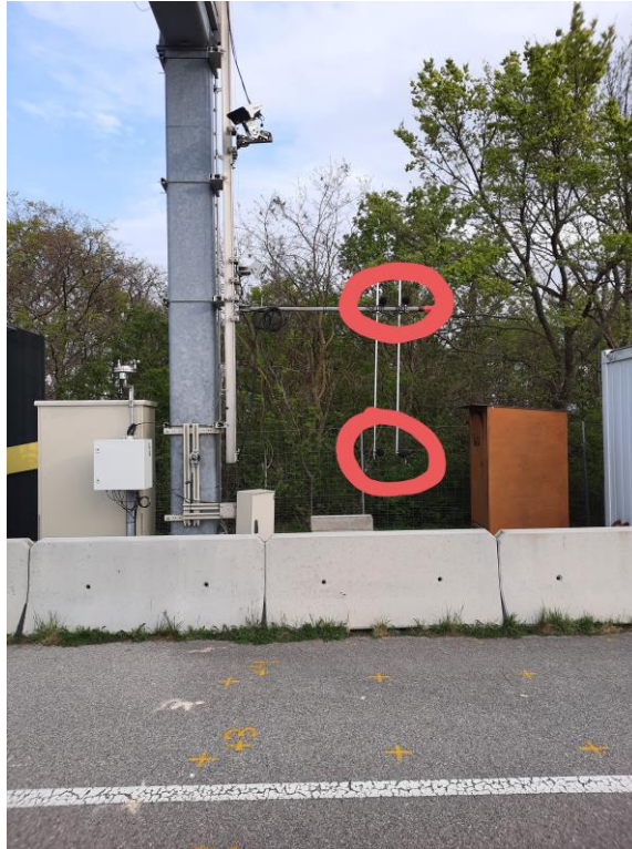
Figure 2: Microphone array with a four-sensor-configuration, horizontal microphone pairs marked in red circles. Note the concrete road barrier that will influence the sound field especially for the lower microphone pair. Test setup in Teesdorf, Austria, April 2022.
