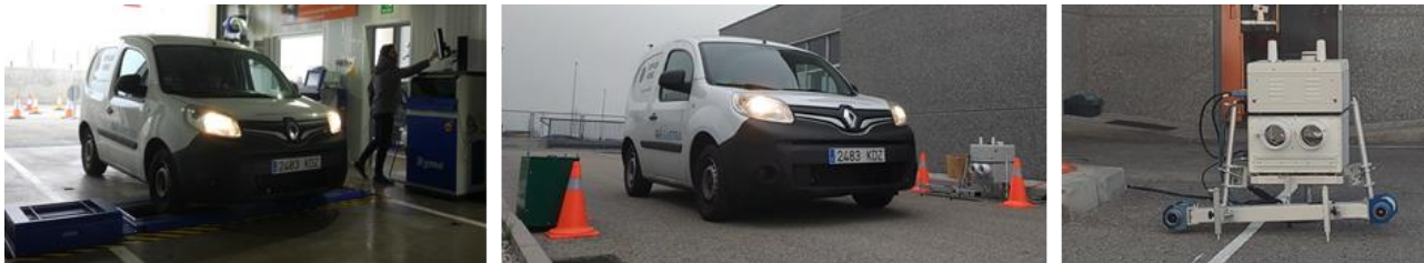
Figure 1. Pictures of the tests performed at the PTI. Left: tests with dynamometer; Middle and right: tests with the RSD.
