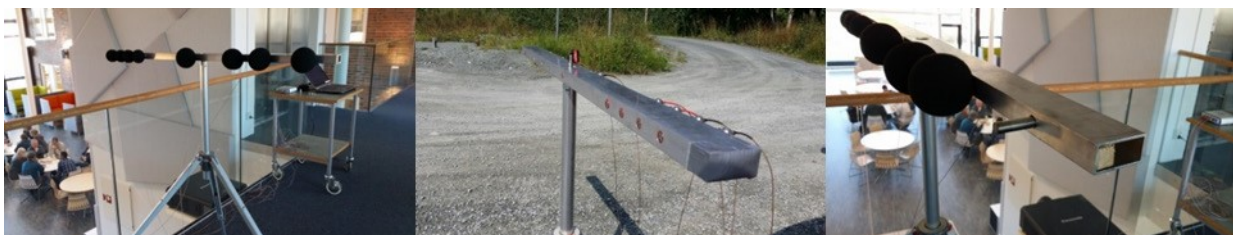
Figure 8: Microphone array used for test
