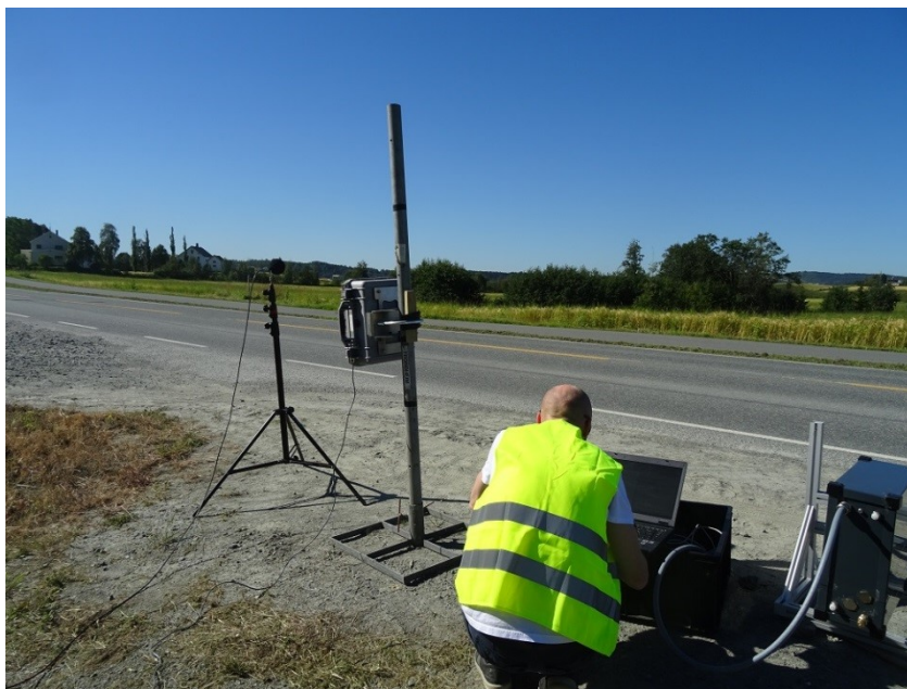
Figure 33: TOPO-bigbox and microphone set-up at Bratsbergveien
